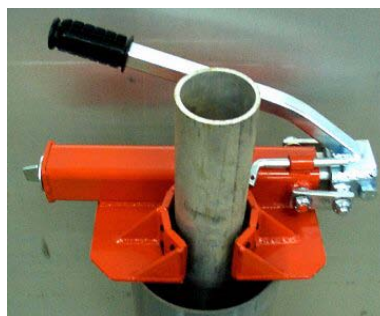
3" steel on 8" casing
