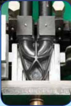
Contractors can now eliminate the time-consuming chore of fusing pipe to fittings. Coils of geothermal Cenfuse pipe are securely fused to the Centennial Bullet™ U-Bend fittings in a climate controlled environment within the Centennial Plastics manufacturing facility. The result is the exclusive Centennial EarthLoop™, which is ready to install the moment it arrives at the job site.
